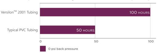
The performance of tubing in peristaltic pumping applications is affected by the conditions of use and equipment utilized, along with the size and wall thickness of the tubing tested. The data above is presented for information only and should not be utilized for specification purposes.
