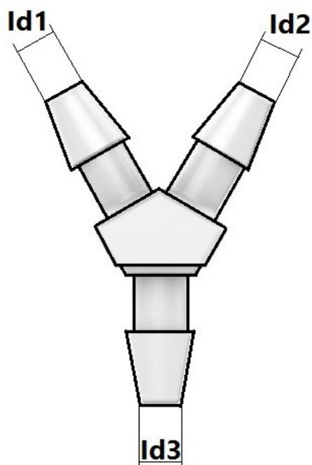
The soft Tubing's are stretched by sliding it over the barbed sides in the right dimensions. They are fixed on the connector due to their self-equilibrating stress of the soft tubing material. For more stability of the connection use an extra clamping piece to fix the tube. A solid, form-fit, leak-tight and removable Y-connection with low dead volume is the result.
